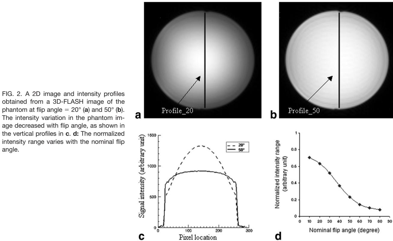
FIG. 2. A 2D image and intensity profiles obtained from a 3D-FLASH image of the phantom at flip angle = 20° (a) and 50° (b). The intensity variation in the phantom image decreased with flip angle, as shown in the vertical profiles in c. d: The normalized intensity range varies with the nominal flip angle.
