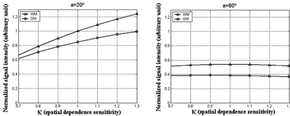
FIG. 1. Simulated FLASH image signal intensity changes with  $\kappa$  in the range of 0.7–1.3 for TR = 45 ms in GM ( $T_1 = 1286$  ms,  $\rho_0 = 0.69$ ) and WM ( $T_1 = 788$  ms,  $\rho_0 = 0.61$ ) at 3T. The intensities were normalized by the WM intensity at  $\kappa = 1$ , and nominal flip angle = 20°. The signal intensity changes very slowly when the flip angle is 60°.
