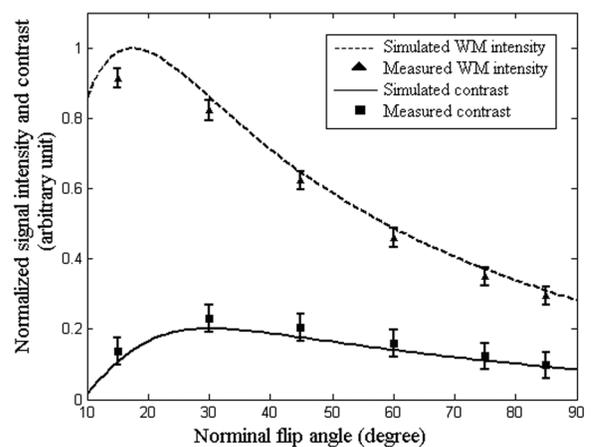
FIG. 4. Simulated contrast and measured contrast of FLASH image as a function of nominal flip angles with TR = 45 ms in GM ( $T_1 = 1286$  ms) and WM ( $T_1 = 788$  ms) at 3T. The simulated contrast assumed a  $\kappa$  of 1.10. The measured signal in WM is also plotted vs. nominal flip angle, and compared with numerical calculations.
